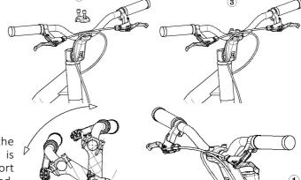
6.2 **Position the stem**. The height of the stem on the M10 model is adjustable. Once the scooter is assembled, adjust its height to provide most comfort and ensure the components are properly tightened. To do this, loosen the screw on the axis (1) and the screw on the lower part of the power arm (2), then place in the desired position, and ensure all screws are properly tightened.
