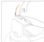
Use a Phillips-head screwdriver to Press down firmly on the edges of Use a Phillips-head screwdriver the bottom. Be careful not to plug into place. pinch any wires.
