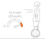
Do not accelerate when the One S1 tilts back or sounds an alarm. Do not attempt to override the speed limiter.
