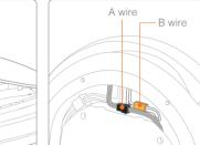
Unplug the black wire (A) first, Pull the connector firmly. Do not pull on the wire itself or you may damage it.
