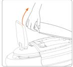
Power off the vehicle and Use a Phillips-head screwdriver disconnect the charger. Then to remove the two screws. Then, then unplug the yellow wire (B). remove the rubber plug on the with a firm tug, use your hand to lift and remove the battery cover.
