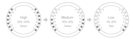
The battery charge level display appears when the One S1 is kept stationary.
