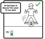
After draining the battery under a 95% charge, the battery is ready for regenerative braking.
