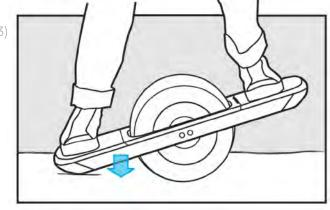
Lower the tail. Once your board is disengaged, slowly lower the tail to the ground.
