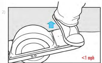
**Lift your heel.** Lift your front heel off one side of the sensor pad and the board will disengage letting you set the tail down.
