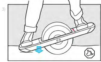
**Lean back and lower.** SLOWLY lean back, the board will travel backwards a couple inches then disengage and the tail will lower to the ground.
