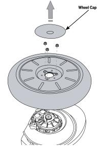
Figure 68: Remove the Tire/Wheel Assembly
