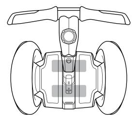
Figure 19: Controller Board Location
