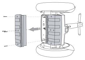
Figure 66: Remove the Batteries
