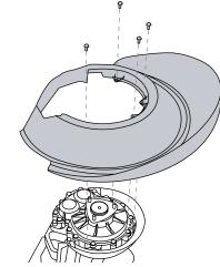
Figure 70: Remove/Install the Fenders
