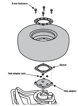
Figure 74: x2 SE Turf Tire/Wheel/Spacer/Hub Adapter
