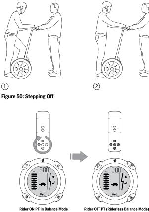
Figure 51: Transitioning to Riderless Balance Mode (Stepping Off)
