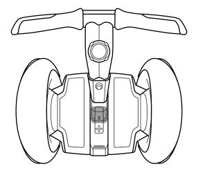
Figure 21: Balance Sensor Assembly Location
