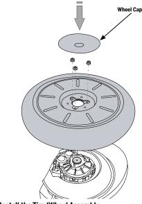
Figure 69: Install the Tire/Wheel Assembly
