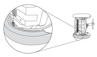
Figure 67: i2 SE Valve Stem Location
