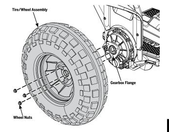
Figure 71: Remove/Install the x2 SE Tire/Wheel Assembly
