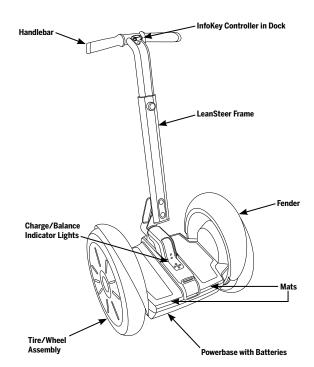
Figure 14: Segway PT Components
