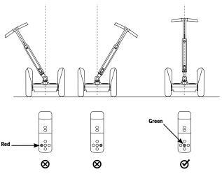
Figure 42: Ensure Balance Indicator is Green
