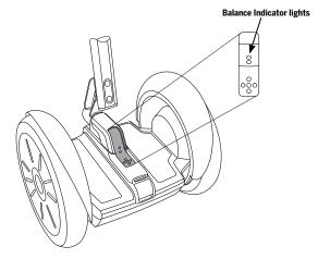
Figure 40: Balance Indicator Lights
