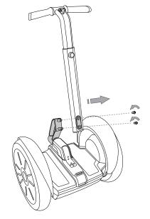
Figure 64: Remove LeanSteer Frame Fasteners
