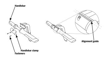
Figure 4: Attach the Handlebar
