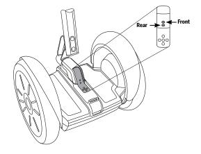
Figure 17: Battery Charge Indicator Lights
