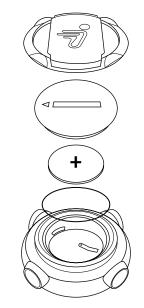
Figure 76: Replacing the InfoKey Controller Battery
