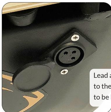
Lead acid batteries can be connected to the Charging socket of the scooter to be loaded!
